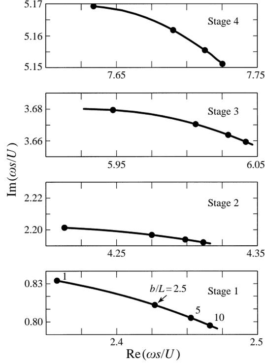
FIGURE 12. Poles of  $D(\omega)$  in the upper half-plane for the first four shallow-cavity operating stages ( $L = 2s$ ).
