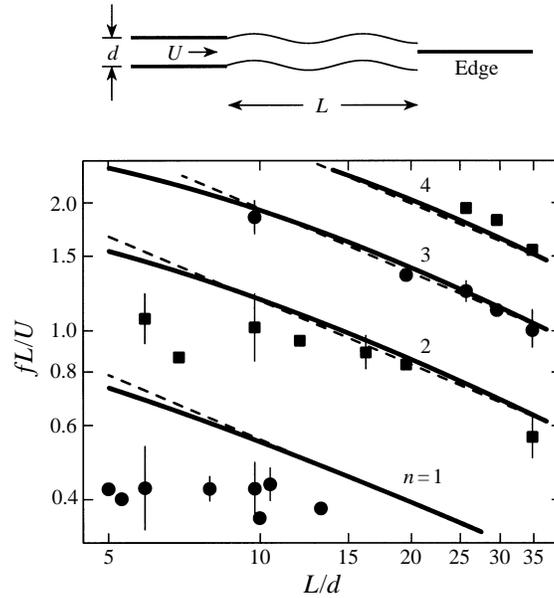
FIGURE 8. Comparison of Strouhal numbers  $fL/U \equiv \text{Re}(\omega s/\pi U)$  from figure 7 — for two-dimensional jet-edge interactions with representative averages of data from Holger *et al.* (1977). The broken lines are predictions of (3.18).
