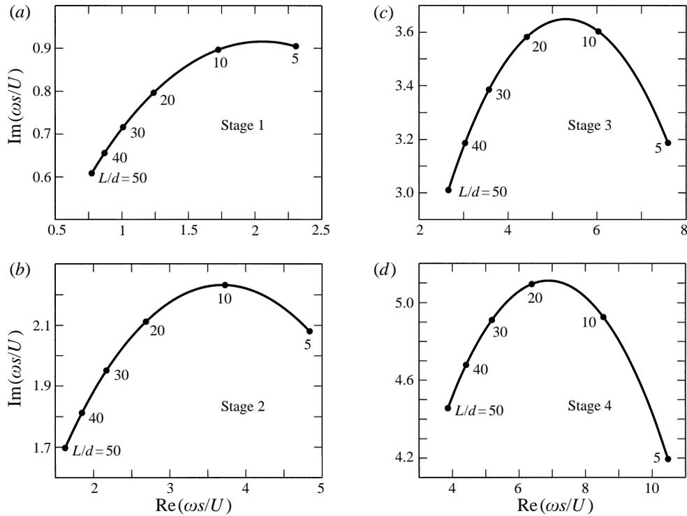
FIGURE 7. Predicted dependence on  $L/d$  ( $L = 2s$ ) of the two-dimensional, jet-edge interaction poles for the first four operating stages.
