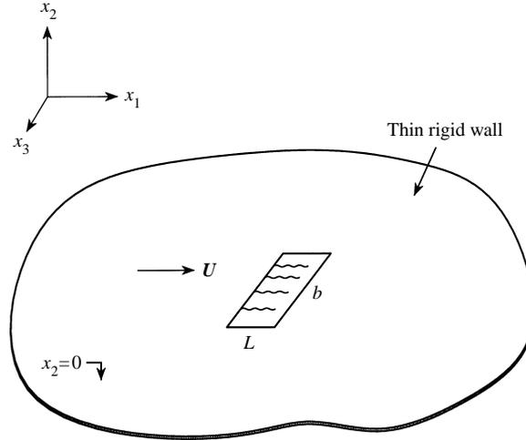
FIGURE 1. One-sided uniform flow over a rectangular aperture in a thin wall ( $L = 2s$ ).
