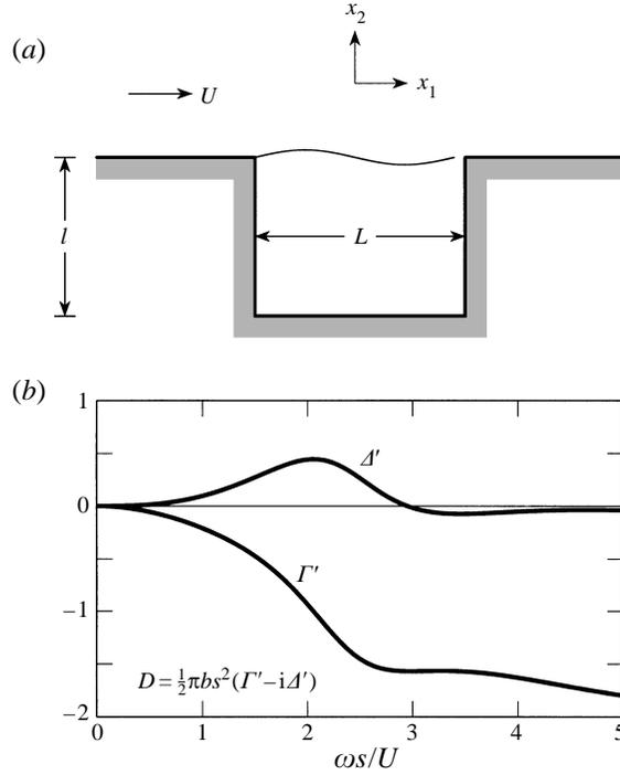
FIGURE 11. (a) Rectangular wall cavity. (b) Real and imaginary parts of the drag coefficient  $D(\omega)$  defined by (4.3) for real  $\omega$  when the cavity aspect ratio  $b/L = 1$  ( $L = 2s$ ).
