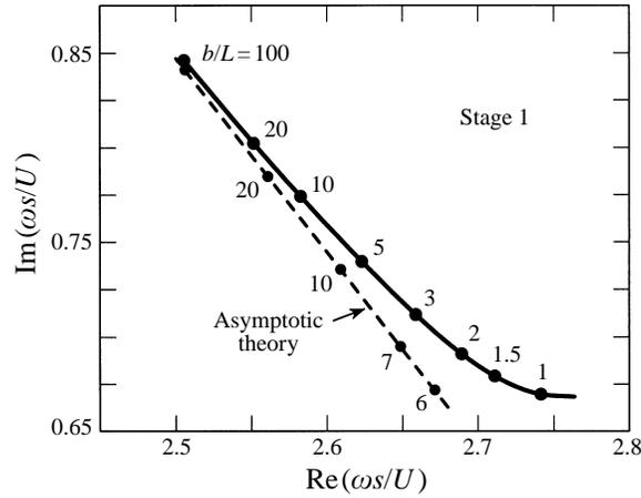
FIGURE 2. Dependence of the first stage pole on aspect ratio  $b/L$  ( $L = 2s$ ) for a rectangular aperture in a thin wall: —, determined by the numerical solution of equation (2.6); - - - - -, determined from the asymptotic formula (2.8).
