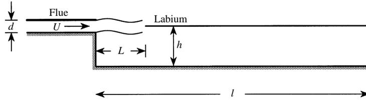
FIGURE 10. Schematic flue organ pipe.
