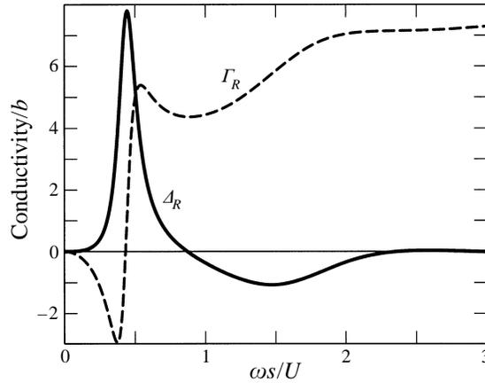
FIGURE 5. Rayleigh conductivity  $K_R(\omega)/b \equiv \Gamma_R(\omega) - i\Delta_R(\omega)$  for a thin jet–edge interaction when  $L/d = 20$ ,  $b/L = 0.5$  ( $L = 2s$ ).
