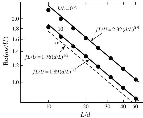
FIGURE 6. Dependence on  $L/d$  ( $L = 2s$ ) of the real part of the stage one pole of the jet–edge interaction for different aspect ratios  $b/L$ : ●, prediction of (3.4); the straight lines are best fits of the formula (3.7) for  $L/d > 20$ .
