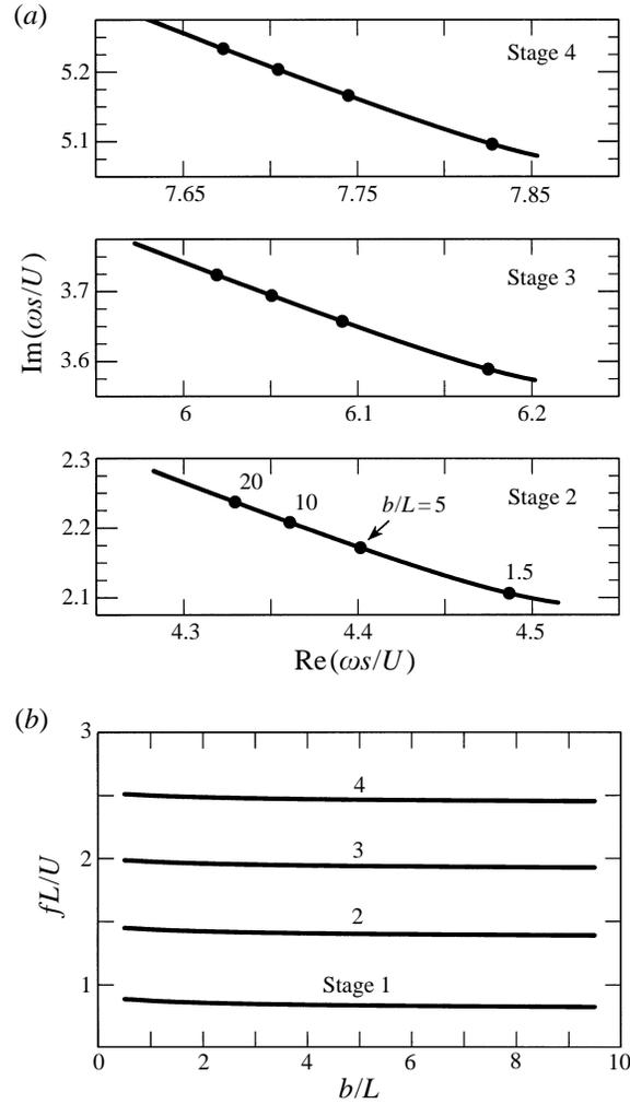
FIGURE 3. (a) Locus of the instability poles in stages 2–4 for a rectangular aperture in a thin rigid wall calculated from the numerical solution of equation (2.6). (b) Predicted dependence of the Strouhal number on aspect ratio ( $L = 2s$ ).
