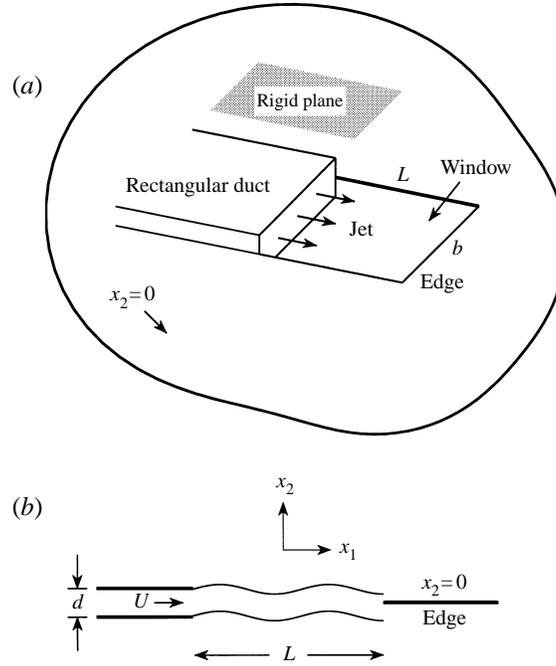
FIGURE 4. Thin, rectangular jet impinging on an edge ( $L = 2s$ ).
