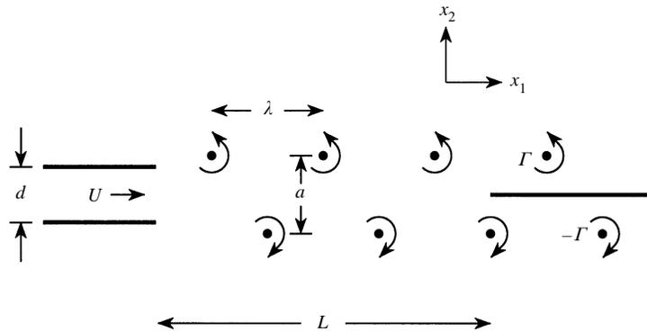
FIGURE 9. Discrete vortex model of the jet-edge interaction.
