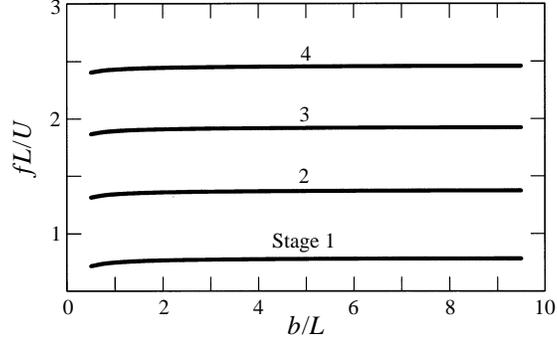
FIGURE 13. Predicted dependence of the shallow cavity Strouhal number  $fL/U$  on aspect ratio  $b/L$  ( $L = 2s$ ) at infinitesimal mean flow Mach number.
